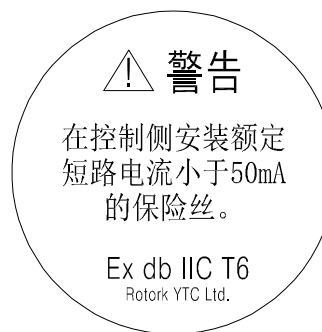
Fig. L-11 : YT-1000 Ex db mb IIC T6 Gb (CCC, NEPSI) (Explosion proof code B of 2.4.1 & 2.4.2 Product Code)
