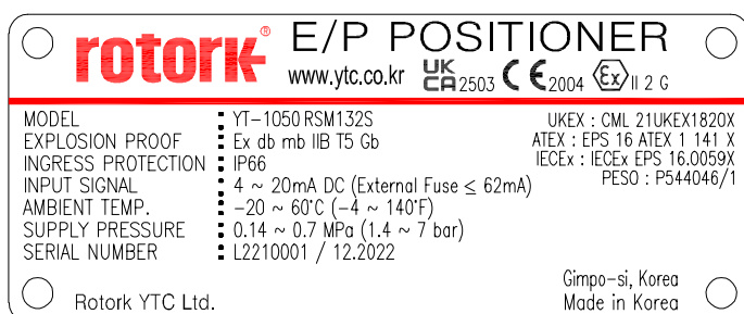
Fig. L-22: YT-1050 Ex db mb IIB T5 Gb (UKEX, ATEX, IECEx, PESO) (Explosion proof code M of 2.4.3 Product Code)
