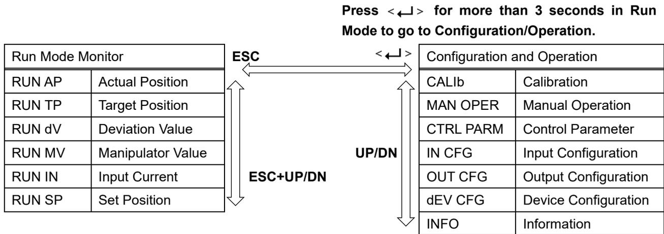
Press the <↵> button to select the lower menu of the Configuration/Operation menu. Press the ESC button to return to parent menu after completing configuration. Pressing the ESC button anywhere in the menu structure several times returns the user to the uppermost menu, Run Mode Monitor menu.
