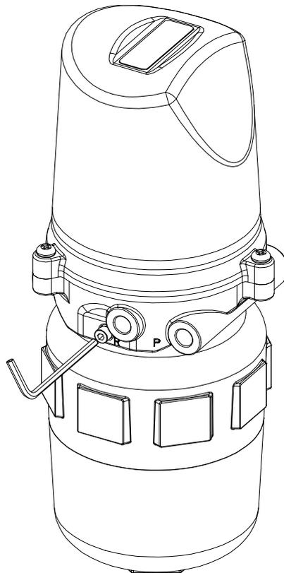
Fig. 3-5: TMP-3000 Fixing the Body
