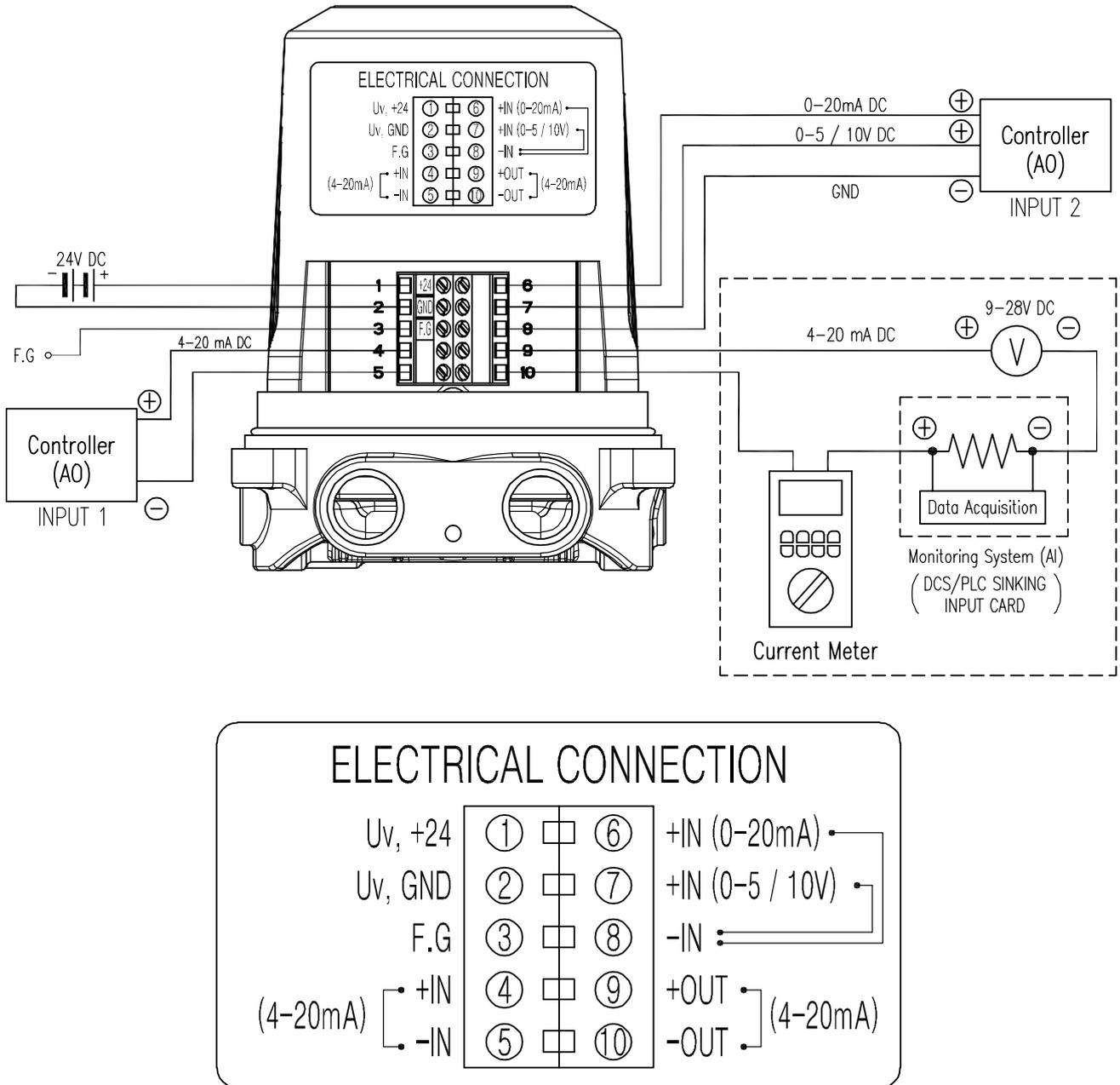
Fig. 7-2: Setting 4-20 mA Analog Output
