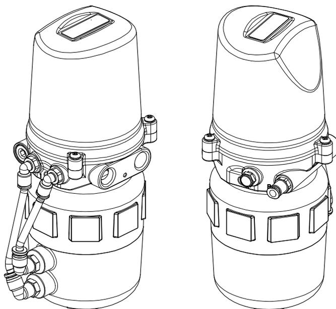
Fig. 4-2: Double Acting Actuator Pneumatic Piping Example
