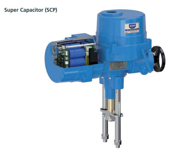
The SCP specification incorporates a super capacitor device inside the actuator, so that when power is cut off, it operates in the open/closed/stop position set by the user, and can be used semi-permanently with a battery or other capacitor storage device.
