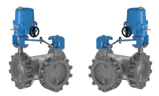
3-WAY butterfly valve used to change the flow direction of fluid or control temperature and pressure. It can be configured with one inlet and two outlets or two inlets and one outlet and is used to distribute or combine fluids and is used when controlling two valves with one actuator. Large size production is possible, and production is possible according to the desired fluid flow direction. Mainly used for cooling and heating control in buildings.
