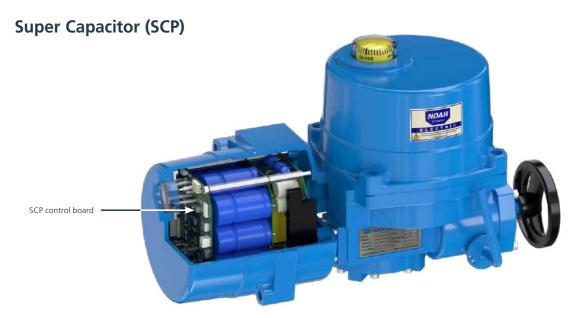
The SCP specification incorporates a super capacitor device inside the actuator, so that when power is cut off, it operates in the open/closed/stop position set by the user, and can be used semi-permanently with a battery or other capacitor storage device.
