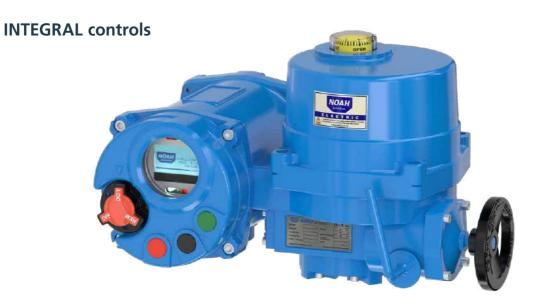
The NA range INTEGRAL actuator can be operated on-site with the integrated operation panel featuring LOCAL/REMOTE selection switch and the open/close/stop buttons. The current operating status can be easily seen on the clear 0~100% LCD. Additional options and control cards can easily be inserted inside the INTEGRAL control unit. It can also be used with all power sources.
