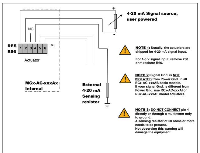
The actuator 4-20 mA output is internally supplying the signal current and can drive sufficient voltage for any sensing resistor of up to 250 ohms.
