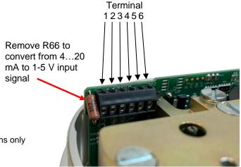
If the sensing resistor R66 is removed, we recommend placing a 10K resistor between signal and signal GND, or simply using shielded cables (for noise reduction).
