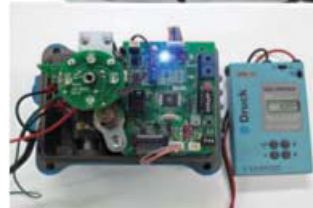
(4mA: Close, 20mA: Open) 4-20mA INPUT (ACTUATOR Operation)
