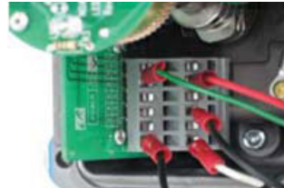
Check the resistive value of PIU (The resistant value when closed: 80~120Ω)
