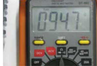
Check the resistive value of PIU (The resistant value when closed: 80~120Ω)
