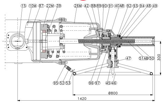
Springs only in SR execution. Otherwise the drawing shows a DA actuator in "open" position.
