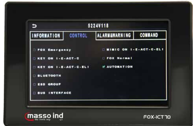
4. CONTROL PRIORITY ACTIVE on VALVE
