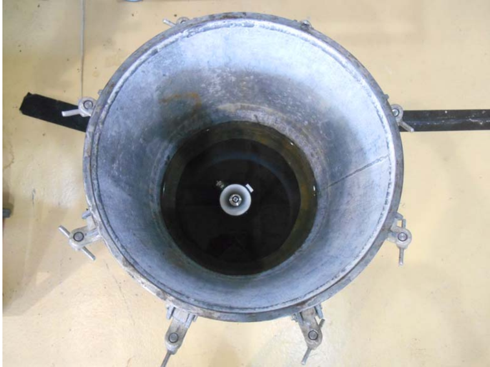
IPX8 INGRESS PROTECTION - PRESSURE CYLINDER – SPECIMEN CONFIGURATION
