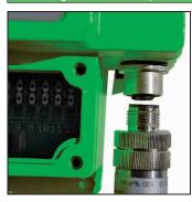
For mounting the sensor must be plugged into the socket and screwed on the sensor by turning the lower knurled screw clockwise. Tighten hand-screwed only.
