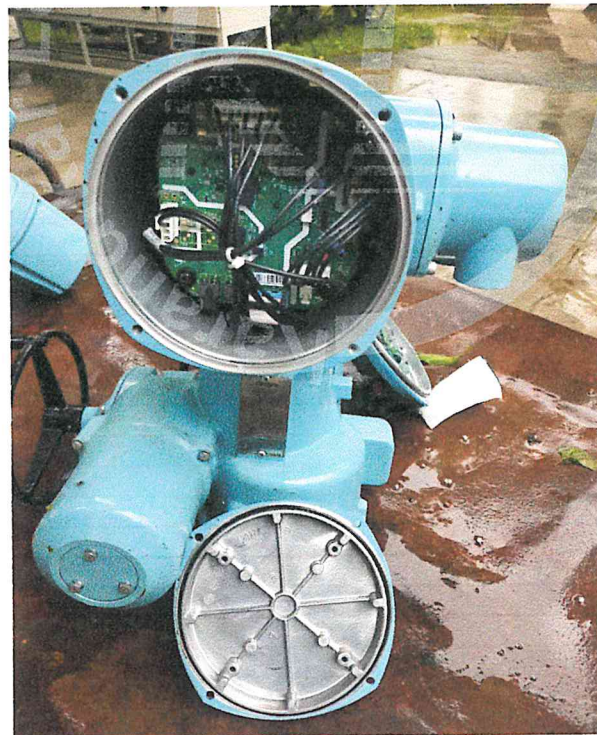
Pictute2: No ingress of powder & water observed
