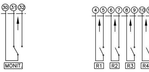
\* Monitor relay can be configured for faults only and will ignore the local control status.
