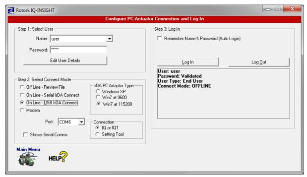
Checkboxes should reflect the equipment in use. Win7 at 115200 should be used by default with Rotork IQ and IQT actuators. Win7 at 9600 can be used if 115200 proves unreliable (IrDA header settings will need to be set for 9600 baud). Communication port settings must match the COM port assigned to the IrDA header in Device Manager.
