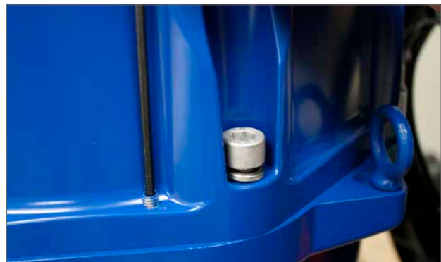
Fig 5.12 Set screw location
