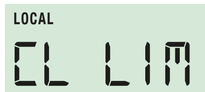
Fig 6.24 Close limit setting
