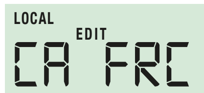
Fig 6.19 Close on force limit
