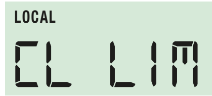
Fig 6.27 Close limit setting
