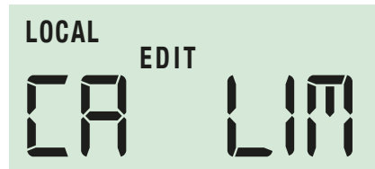
Fig 6.18 Close on position limit
