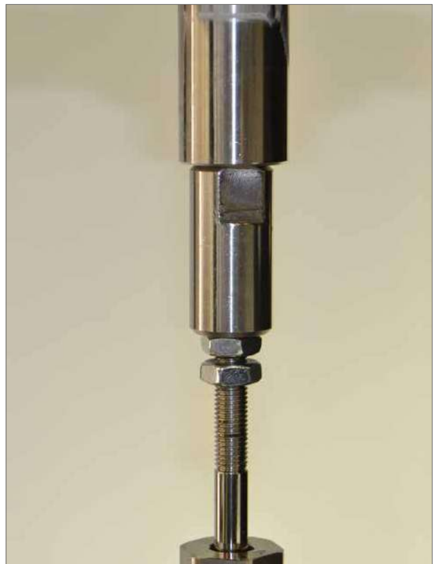
Fig 5.7 Connection of valve shaft and actuator shaft
