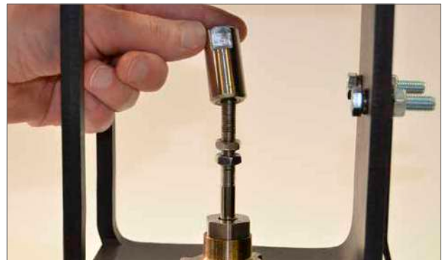
Fig 5.4 Coupling attachment to valve shaft
