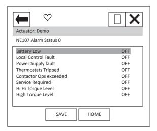
'Battery Low' indicates that the actuator battery used to maintain the display, is either flat or low.
