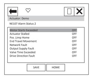
'Motor Starts Exceeded' indicates that the limit for the number for motor starts expected in the actuator life has been exceeded.
