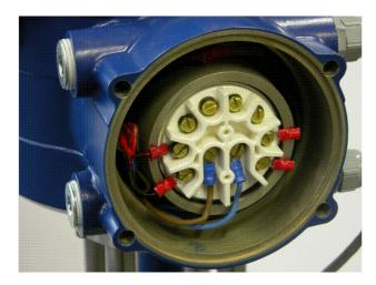
Network connections are made to the terminals of the actuator. Shown above is a typical arrangement for a CVA range actuator. HART is connected to terminals 1 and 2. Always check the actuator wiring diagram for correct terminal numbering and connection polarity.
