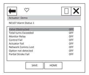
'Valve Obstructed' indicates that the actuator has tripped/stopped on torque due to an obstruction in the valve.
