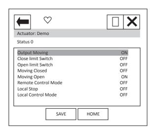
'Output Moving' indicates that the actuator is currently moving.
