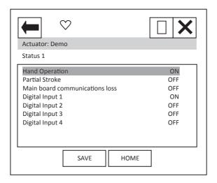
'Hand Operation' indicates that the actuator is currently moving under manual / hand control.
