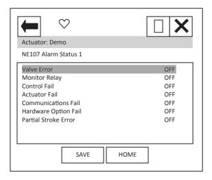
'Valve Error' indicates that the actuator has tripped/stopped on torque due to an obstruction in the valve.
