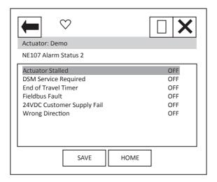
'Actuator Stalled' indicates that the actuator has stalled.
