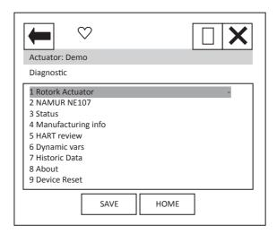
Item 1 indicates the type of actuator. Note, for SI actuators (SI3 and SI4), this will display "Rotork Actuator".
