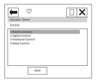
Item 1 'Rotork Actuator' indicates the type of actuator.
