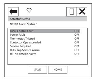
'Local Control Fault' indicates that there is a fault in the actuator's local controls.
