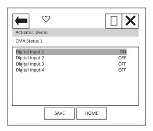
'Digital input x' indicates the status of the actuator hardwired digital inputs.
