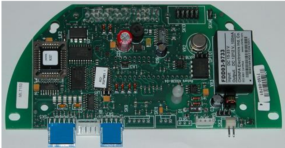
Fig 4: The Interface Card (Q and Skil/EH actuators)
