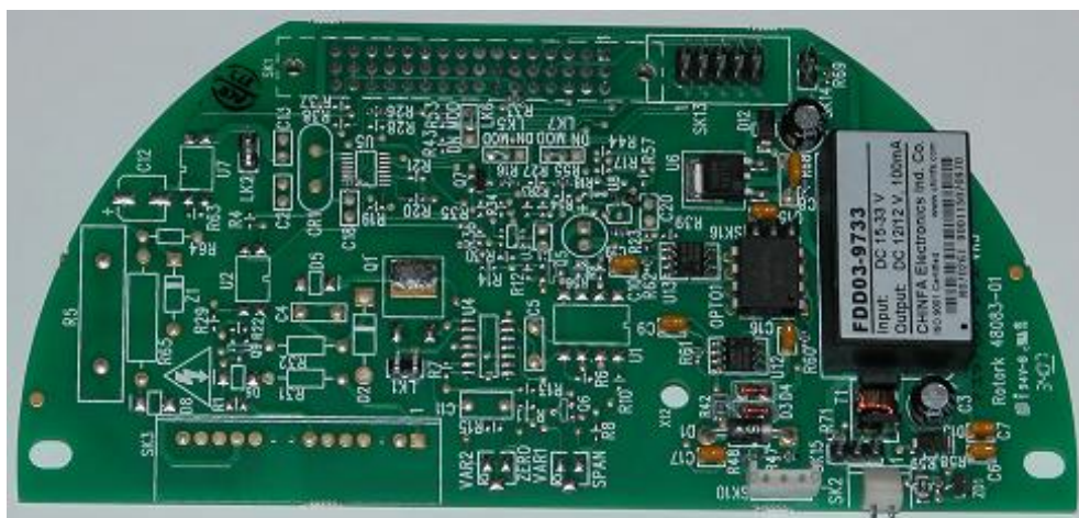
Fig 5: The Interface Card (IQ/IQT actuator)
