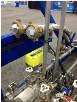
Schischeck ExMax on a process skid
