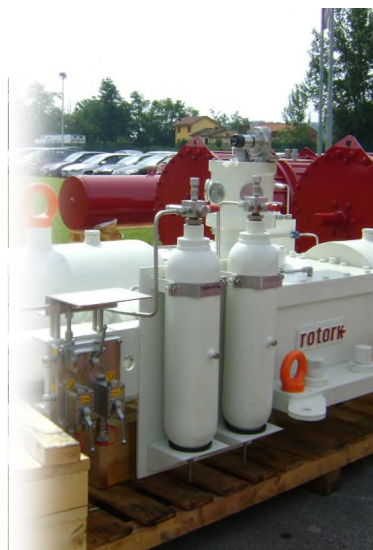
Specialised hydraulic actuator package
