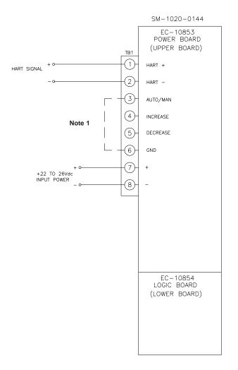
Due to wide variations in the terminal numbering of actuator products, actual wiring should follow the print supplied with the actuator.
