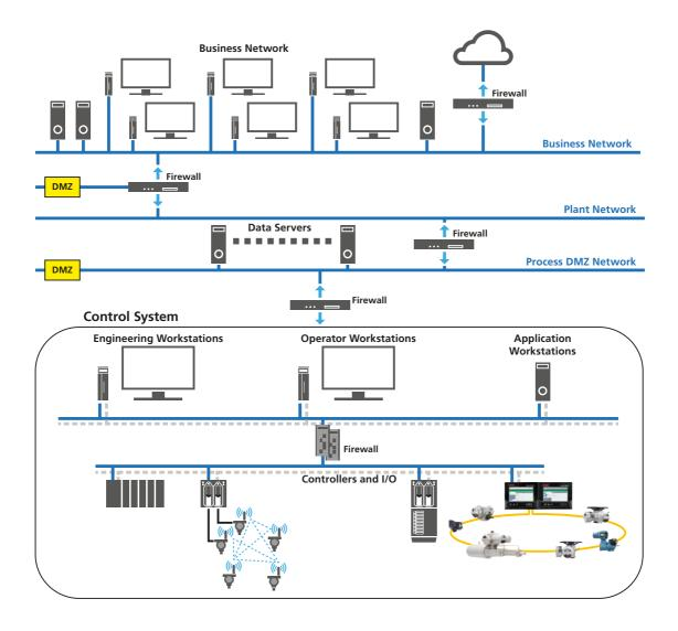
The diagram above shows an example plant with cyber security protection. Segmentation of networks forms separate security zones that are important to protect the control system. Security zones use firewalls and other security devices to only allow authorised network traffic between the zones.
