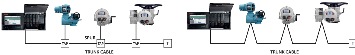
Fig 8.1.1: RS-485 Data Highway Topology – Single Channel
