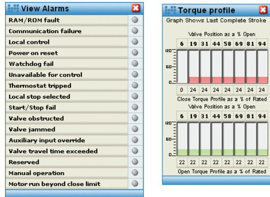
Fig. 23. Alarm and valve torque profile indication
