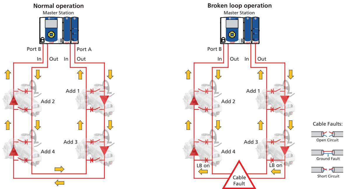
Fig. 7. System fault tolerance - 2-wire loop integrity.
