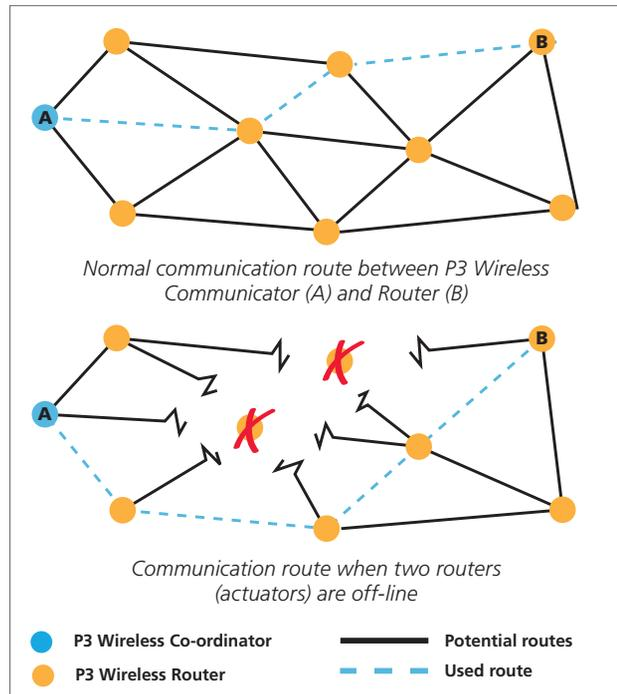
Fig. 12. Explanation of mesh network redundancy paths.
