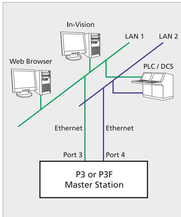
Fig. 27. Multiple ethernet LAN connections
