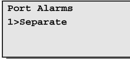
This screen allows port alarm handling to be configured. Alarms can either operate completely independently ('separate') for each port, or can be linked such that the same alarm information is always reported regardless of which serial port is used.
