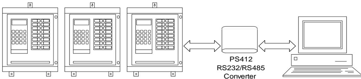
Fig 20: RS485 connections
