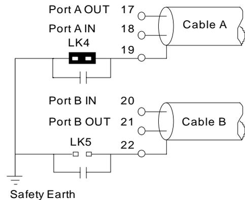
**If there is a signal earth bar** - one of the screens may be connected to the bar in addition to them both connecting to the master station, in this configuration both LK4 and LK5 should be removed.
