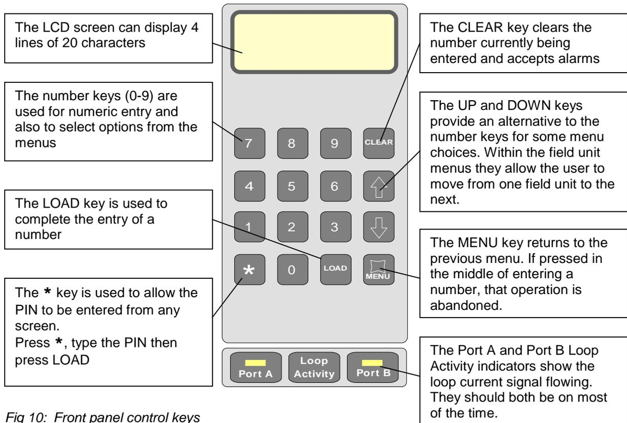
Fig 10: Front panel control keys
