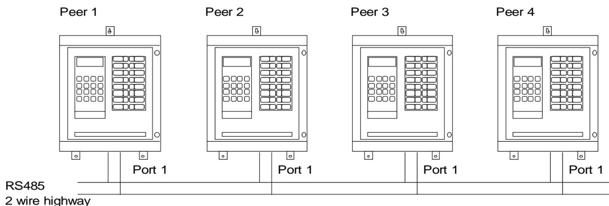
Fig 13: Peer to Peer master station communication
