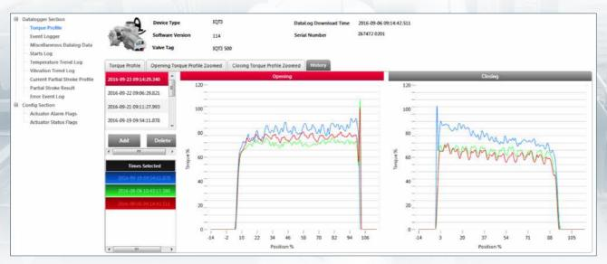
Above: Rotork's intelligent asset management system showing torque data from multiple actuator datalogs.
