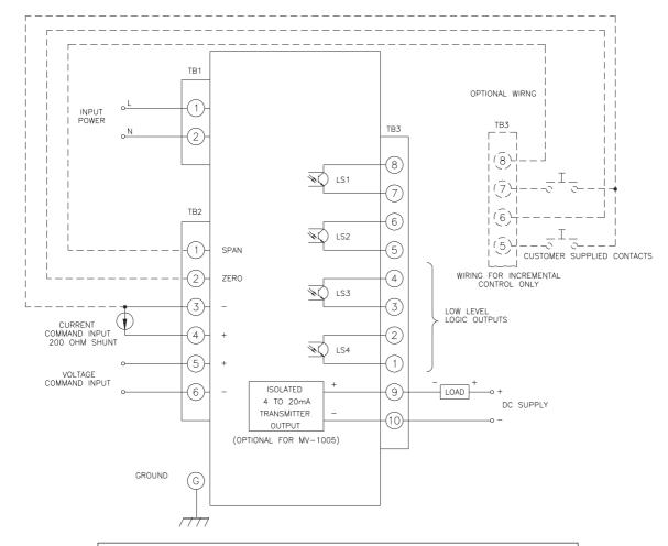
Due to wide variations in the terminal numbering of actuator products, actual wiring of this device should follow the print supplied with the unit.
