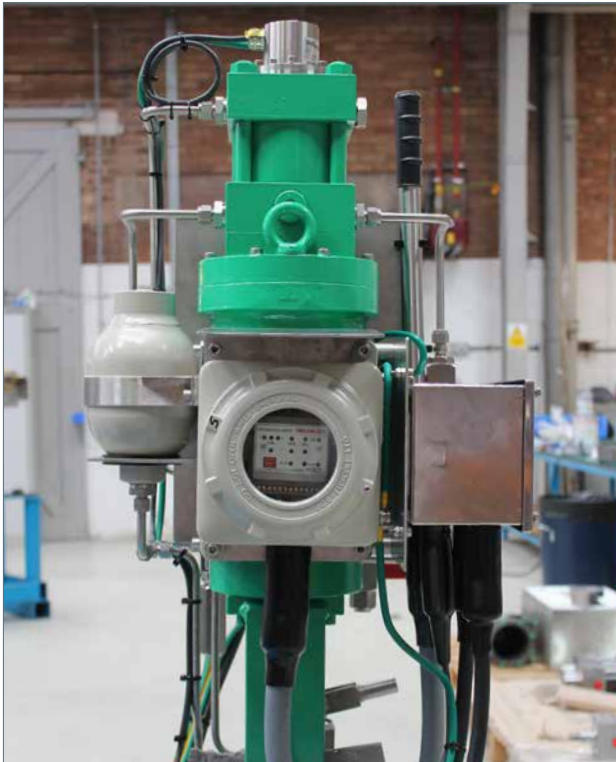
Spring fail (to close) control system
