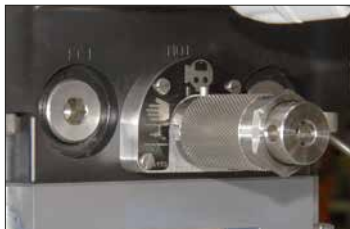
Fig. 6.1.1. Manual Override Handle
