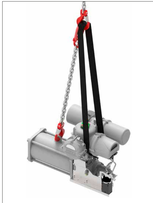
Fig. 4.1.2. SI3 RH Lifting: Slings attached to the lifting eye and controller centre housing.
