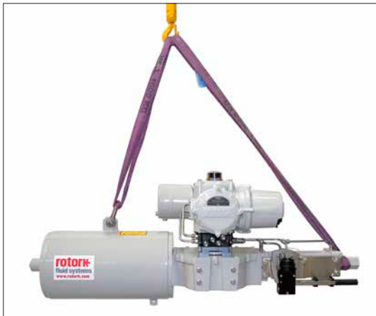
Fig. 4.1.1. SI3 GH lifting: Slings attached to the lifting eye and hydraulic cylinder stop bolt cover.
