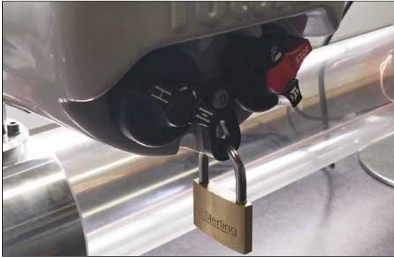
Fig 6.1. IQ / IQT control selector padlocked in "Remote"
