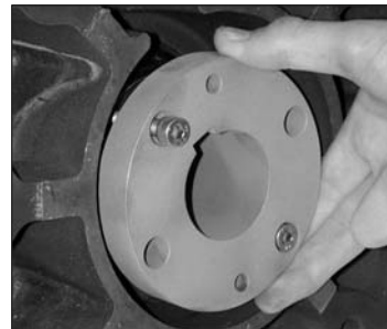
Fig. 4.14 B3/B4 Drive Bush in Situ
