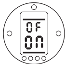
Bus System Positioning Control Screens [ON]
