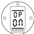
Pakscan Set-up Screens ON
