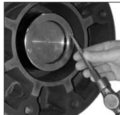
Fig. 4.6 Removal of Retainer
