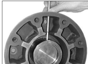
Fig. 4.5 Locating Set Screw
