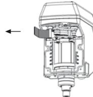
If open cover bracket gear belt is removed from tensions after this choose the right setting acc. to stroke by hand – not use any tools. Due to repeatedly move of the red bar the setting of the gear belt gear can be changed. The position is corrected by closing the cover and starting a re-adjustment drive.
