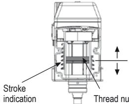
Stroke can be adjusted by thread nut from min 5 mm to 60 mm.
