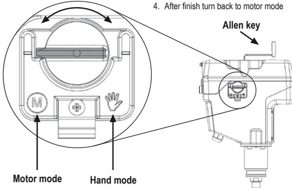
When operating the manual override in case of failure it is possible that the gear decouples. It can be seen that the selector switch is turned on motor, the actuator when controlled does not execute any stroke movement. The blockade is resolved by simultaneously rotating the motor-hand switch and turning the Allen key in the hexagon shaft. The gear engages.
