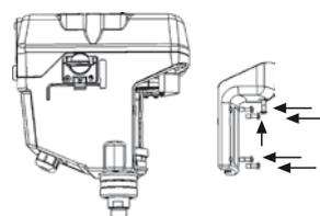
5 × fix screws tighten.
