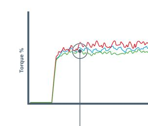
Valve seating, sealing and other mechanical issues can be detected from only subtle changes in torque.
